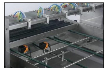
Sensors used to recognise baking trays
