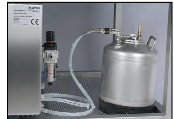
Compressed air connection and 9l oil tank
